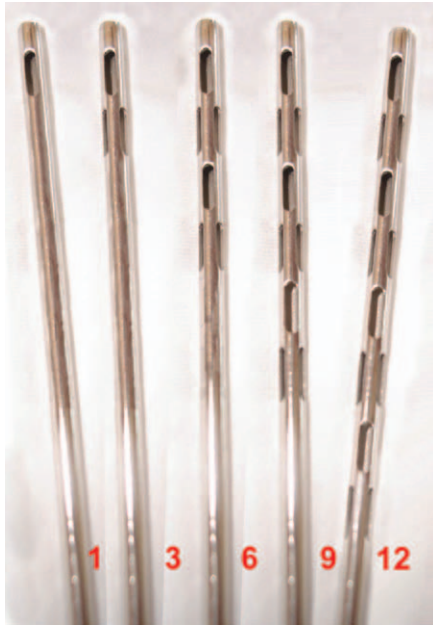
Fig. 2. Five 12-gauge (2.7 mm) cannulas with increasing numbers of 1 × 2-mm holes.
